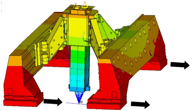
Figure 4: Load case I: acceleration in X-direction at the drives of the traverses.
