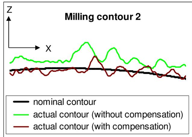
Figure 13: Milled contours at segment 2 (amplified with factor 250).
