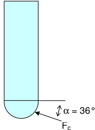
Figure 7: Cutting force acting at a milling tool.
