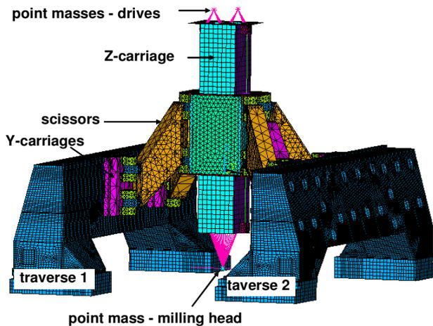
Figure 3: Machine tool “scissor kinematics”.
