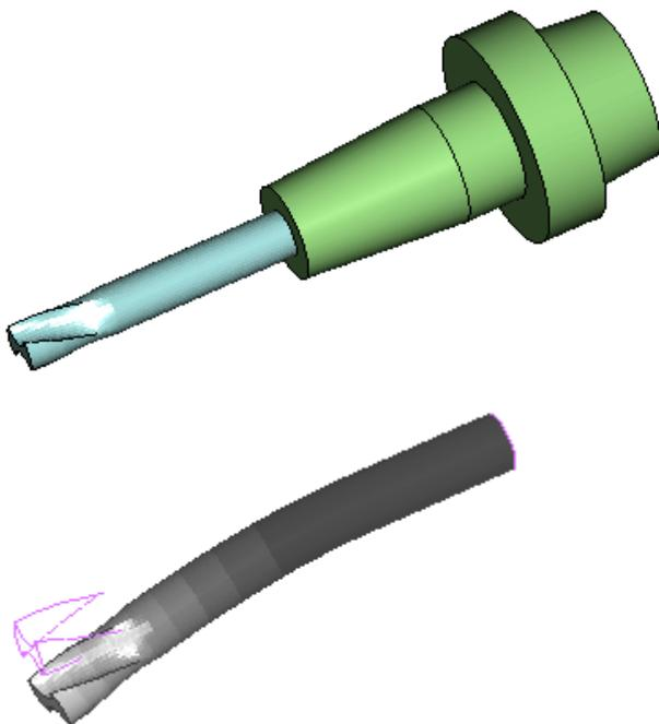
Figure 6: Model and deflection of a milling tool.
