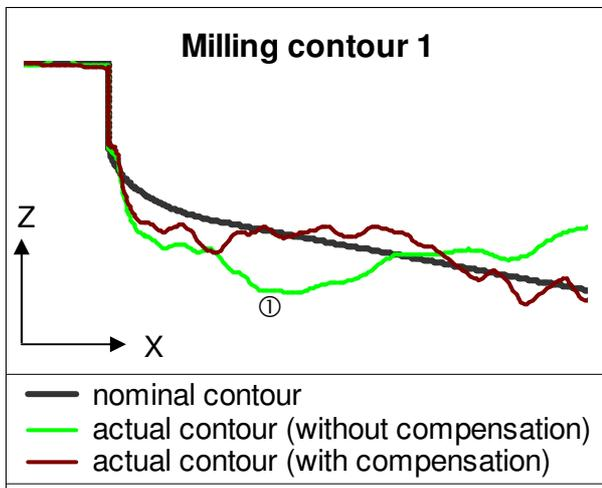
Figure 12: Milled contours at segment 1 (amplified with factor 250).
