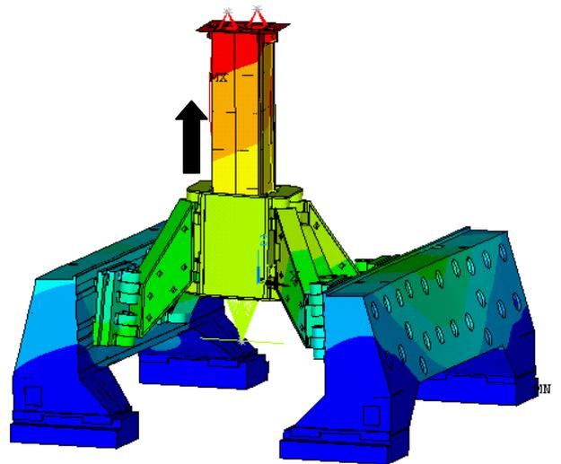
Figure 5: Load case IV: acceleration in Z-direction at the drives of the Z-carriage.
