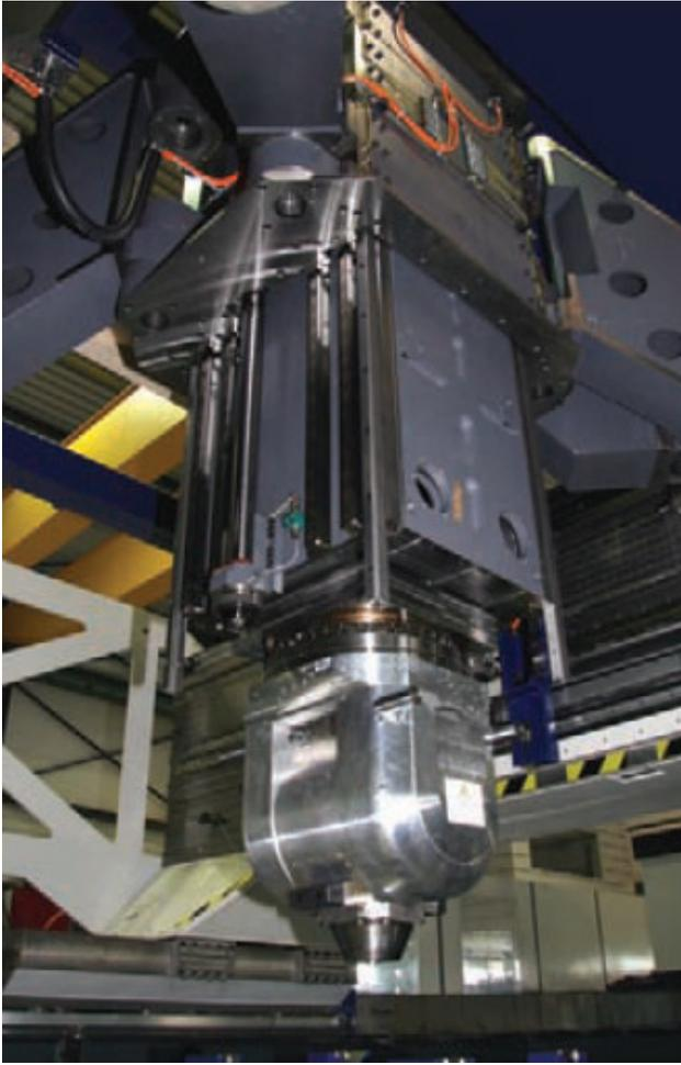
Figure 2: Machine tool with “scissor kinematics”.
