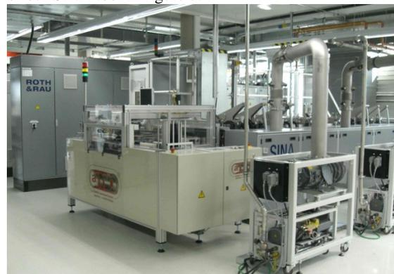
**Figure 7:** Photograph of the Roth&Rau SiNA tool used for the deposition of a-Si layers using an industrial PECVD reactor within this investigation.
