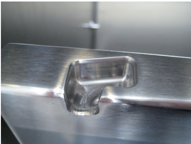
Figure 6. Cut-outs in the shelves fulfil EHEDG Doc. 8 requirements.
