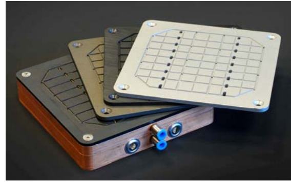
Figure 6: Solar cell mounting chuck for bifacial 5" solar cells with 62.5 mm busbar distance. The changeable surface plates allow the variation and assessment of the surface reflectivity.
