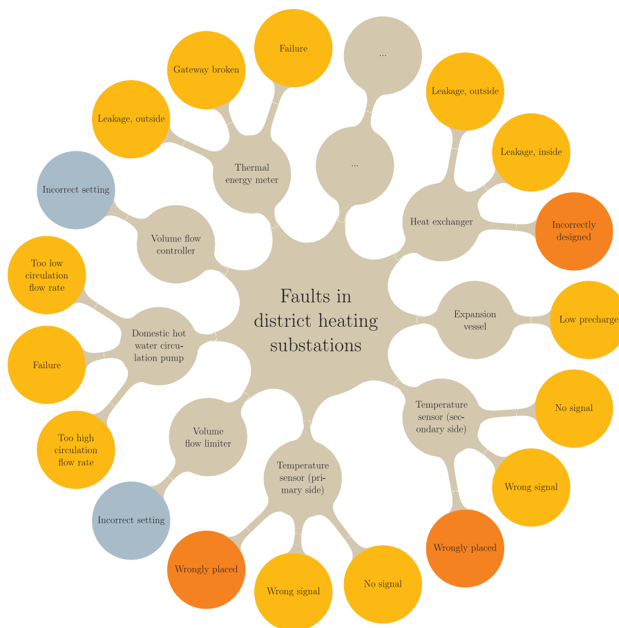
Fig. 2. Excerpt of the faults in substations grouped by the affected component and coloured by fault type.
