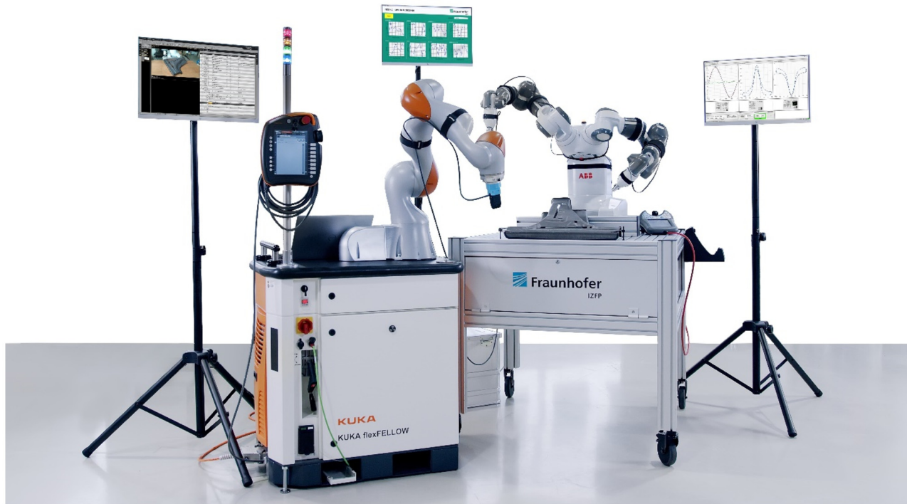
Figure 3: NDE 4.0 demonstrator consisting of a dual robot unit (left: KUKA LBR iiwa, right: ABB YuMi). The B-pillar base is located on the worktable of the ABB YuMi. The three displays show raw data of a sensor (right), the common display of all current sensor results (middle) and the documentation in DICONDE (left).
