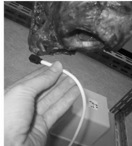
Fig. 4: Measurement of the orientation of the sensor sockets by means of a magnetic tracking system. The transmitting box creates a magnetic field and detects the tip of the magnetic sensor
