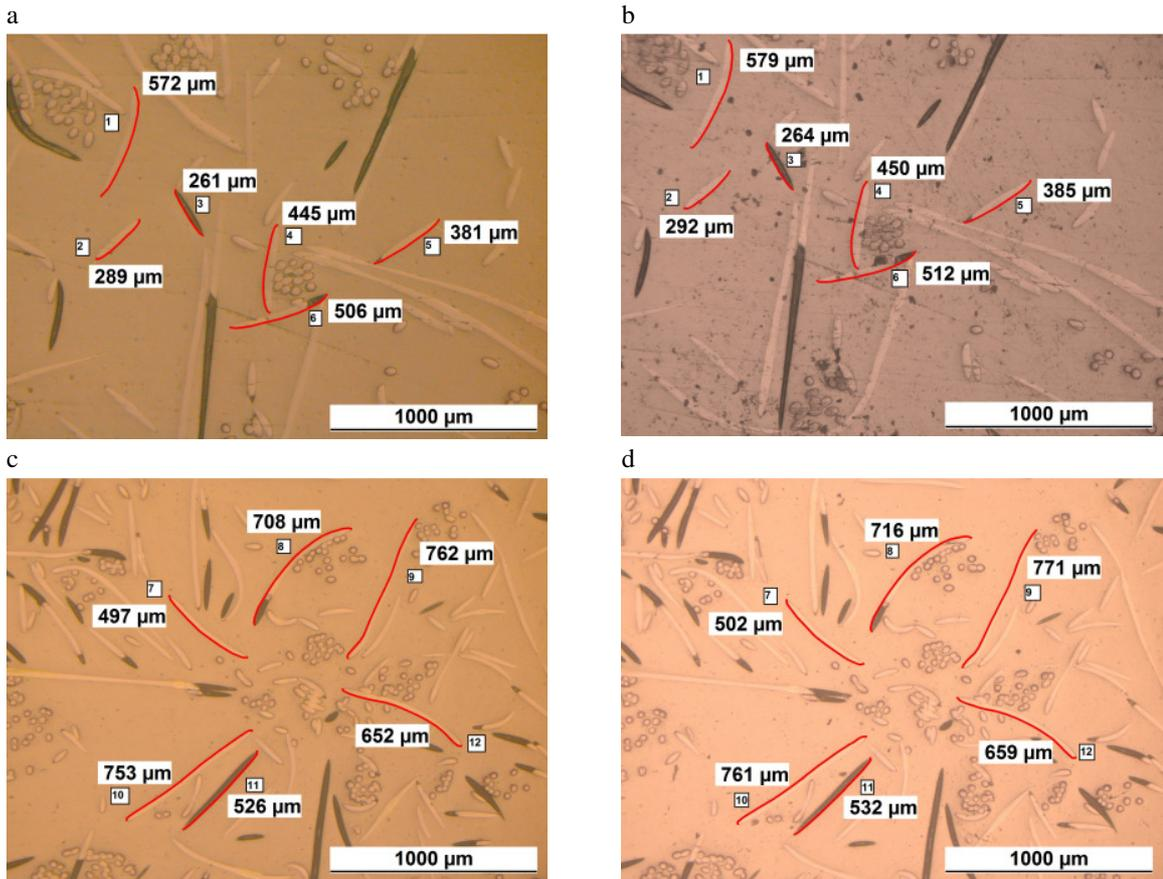
Figure 4. Optic microscopic images of CIPP samples showing surface morphology (a) specimen 1 before aging (b) specimen 1 after 5 weeks aging (c) specimen 2 before aging (d) specimen 2 after 5 weeks aging
