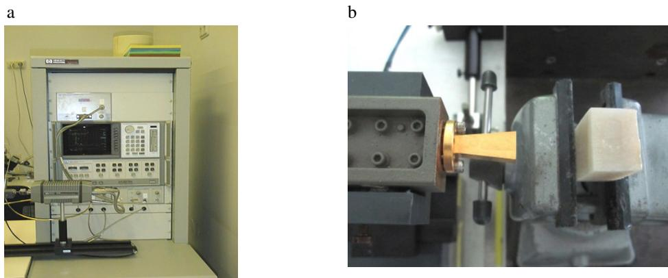
Figure 2. (a) Vector network analyzer with amplifiers and source module. (b) horn antenna and sample with 50 mm distance
