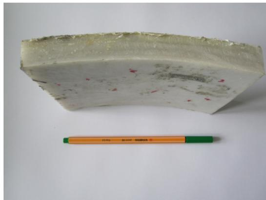
Figure 1. CIPP specimen taken out from a tube
