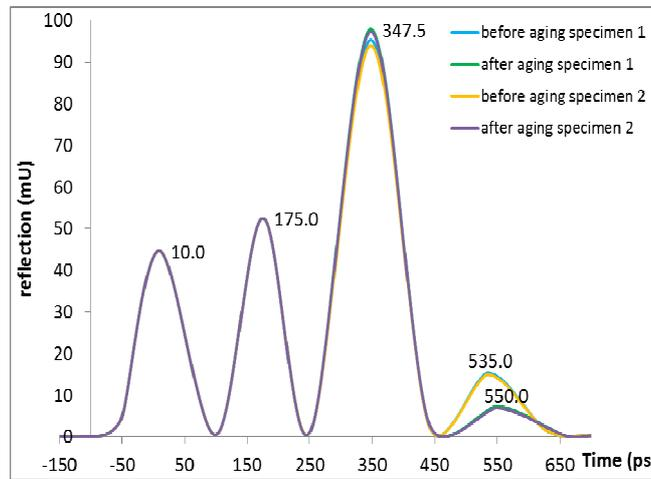
Figure 6. Reflection measurement in time domain mode of specimen 1 and 2. The values are displayed in relative units (U: units; mU: milliunits).
