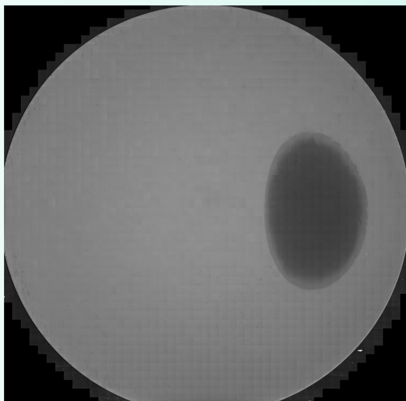
Fig. 1: UV-PL image of epitaxial wafer with observable facet region on the right wafer side
