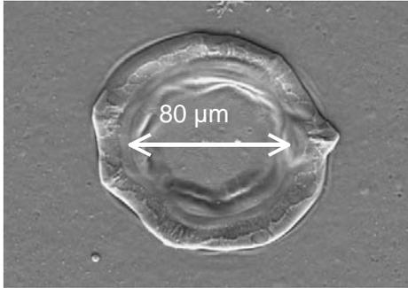
Figure 2: Top view SEM picture of a laser-fired contact.
