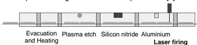
Figure 4: Integrated laser-fired contact production line.
