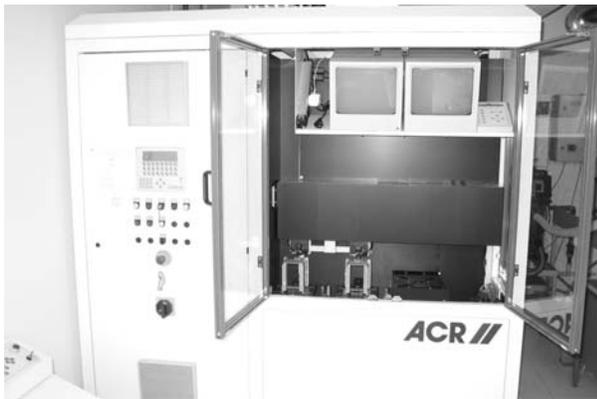
Figure 3: Pilot type scanning laser system with automated wafer handling.
