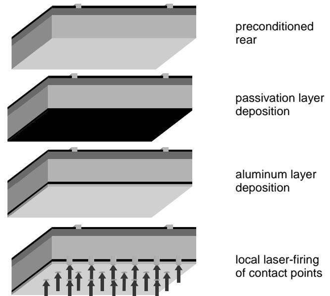
Figure 1: Sequence for the laser-fired contact process.
