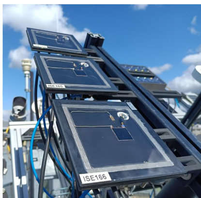
FIGURE 2 Component cell sensor (ISE164, ISE165, and ISE166) adapted from CPV applications for the evaluation of the spectral conditions during outdoor measurements of flat-plate modules. 25
