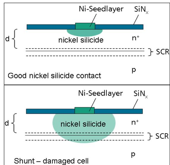
Figure 5: Damaging mechanism of nickel in silicon solar cells
