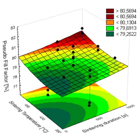
**Figure 6:** Pseudo fill factor after sintering for mask & etch-ablated solar cells for different sintering temperatures and durations.
