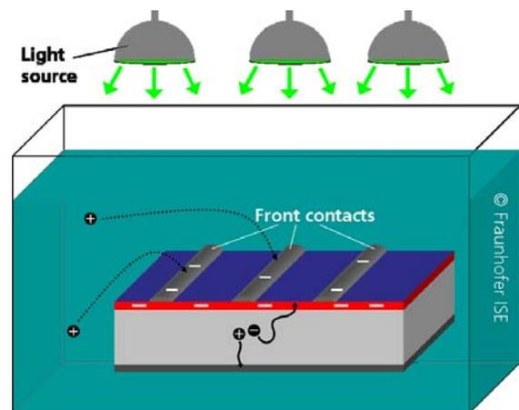
**Figure 3:** Schematic image of the light assisted electroless plating
