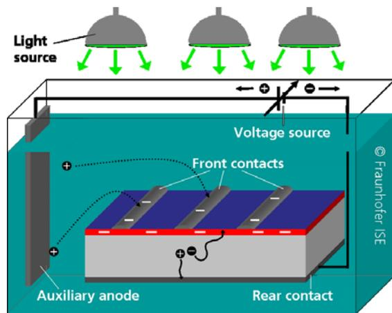
Figure 4: Schematic image of light induced plating
