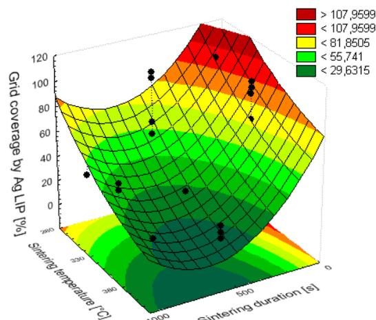
**Figure 8:** Resulting percentage of the grid covered with silver after the subsequent reinforcing step for mask & etch-ablated solar cells sintered at lower temperatures. Values above 100% are artefacts of the statistical model.
