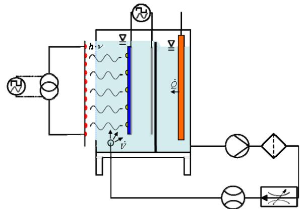
**Figure 2:** Schematic image of the used plating bath setup
