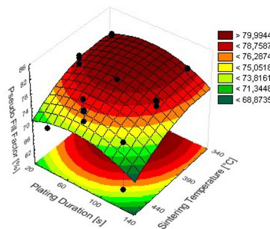
**Figure 9:** Pseudo fill factors of solar cells with laser ablated ARC sintered at different conditions.
