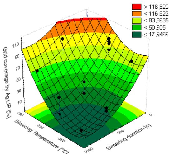
**Figure 10:** Resulting percentage of the grid covered with silver after the subsequent reinforcing step for laser ablated samples. Values above 100% are artefacts of the statistical model.
