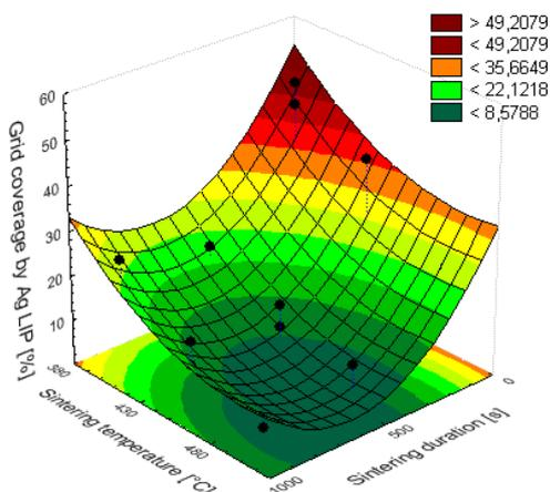
**Figure 7:** Resulting percentage of the grid covered with silver after the subsequent reinforcing step for mask & etch-ablated solar cells for different sintering temperatures and durations.
