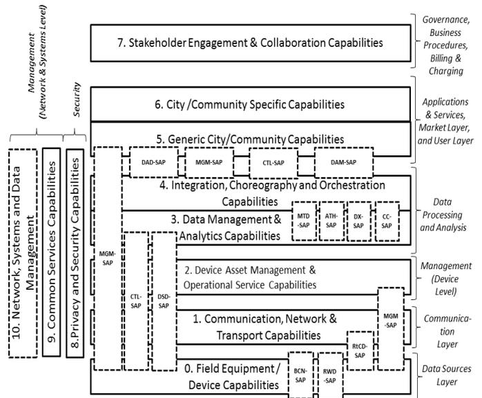
FIGURE 3: THE OUPPLUS ICT REFERENCE ARCHITECTURE FOR ENABLING SMART CITIES
