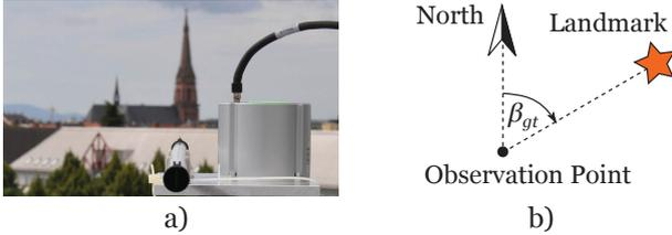
Fig. 4. Establishing ground truth: a) Bearing tube with rigidly attached IMU pointing at landmark: Church spire. b) Ground truth heading  $\beta_{gt}$  given by coordinates of the observation point and landmark.
