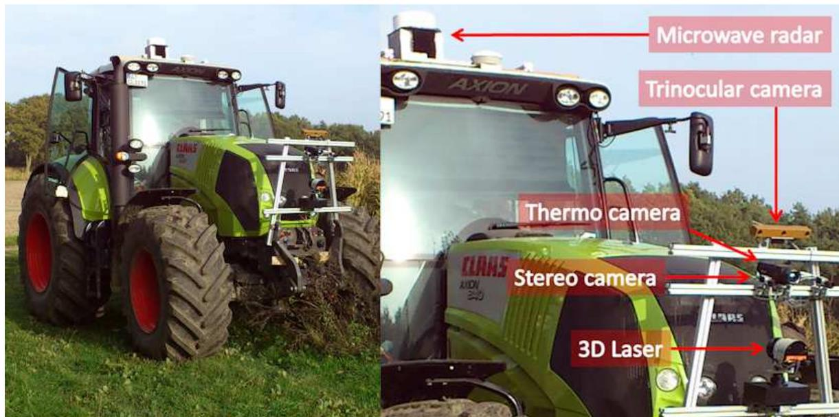
FIGURE 1: Positioning of the sensors on the tractor
