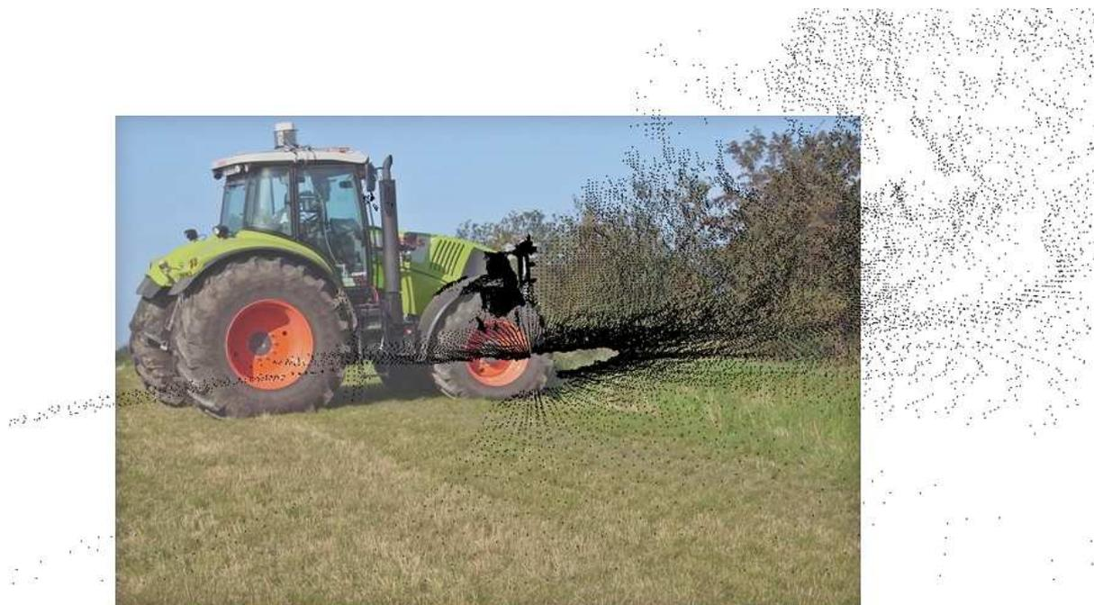
FIGURE 3: Photo composition of a point cloud created by the lidar sensor and a camera image of the corresponding scene.
