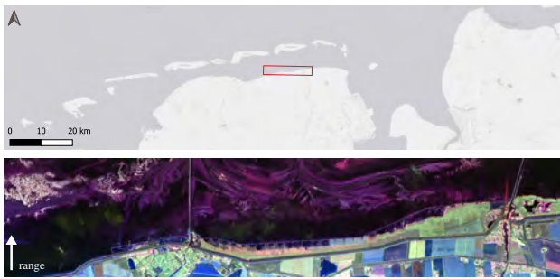
Figure 1. Top: Geographic location of the study site. Bottom: PolSAR image (S-band) color coded corresponding to the Pauli decomposition.
